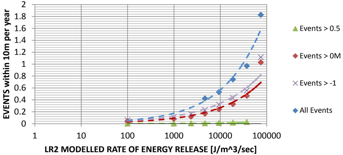
**Figure 3 Correlation between modelled RER and Event occurrence, by Magnitude at an example mine. The correlation is based on over 30000 events measured over 4 years**
