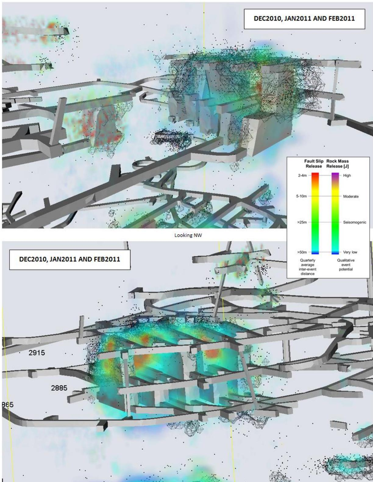
**Figure 4 Modelled Rate of Energy Release versus Seismicity for an example period from NRS mine.**
