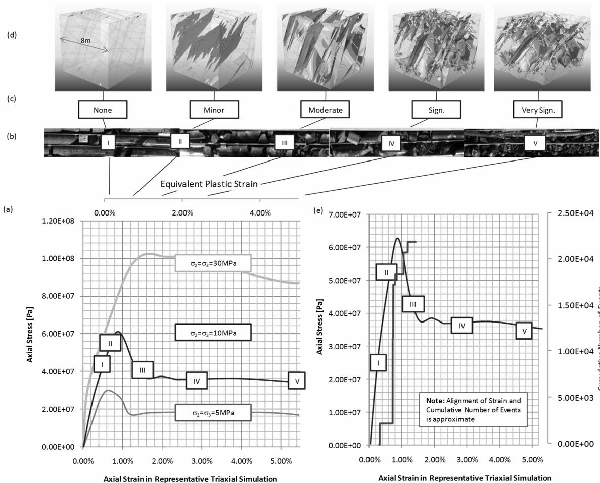
**Figure 2 Comparison of stress-strain-energy release of a simulated rock mass specimen (8m diameter) at varying levels of confinement and photographs of diamond drill core specimens, from locations estimated by calibrated global models to be at these respective states of strain, after Beck et al 2009**
